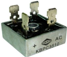
**A solid state bridge rectifier:** This is essentially four (or more) large diodes mounted inside a square metal or epoxy case. These can be purchased for under £5.00 (GBP) from either motorcycle or general electronics vendors (Maplins, Radio Shack ect..) and should be rated at around 100V\20A.
