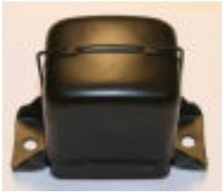
Dynamo equipped machines were generally fitted with a Lucas CVC Dynamo regulator. This unit regulated the voltage by electro-mechanically switching the supply to the battery from the dynamo on and off very fast. These modules need maintenance and have to be set between a maximum charge voltage and a minimum switch off voltage which is always a bit of a compromise. They also have both moving parts and contacts that wear.
